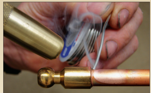
SweatJets are easy to solder using a propane torch.
