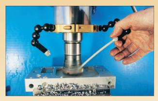
▲ Each **VariFlow** nozzle is infinitely adjustable from full shut off to maximum flow.
