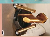
**Brass ExtensionTubes** are ideal for directing coolant straight to the cutting edges.
